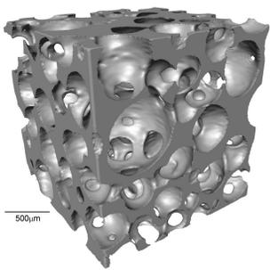
Fig. 4 Micro-CT image of hybrid foam scaffold
