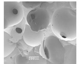
Fig. 3 SEM of bioactive glass foam
