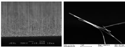
SEM images of 1.7-eV GaAsP nanowires on Si substrate for high-efficiency solar cells
