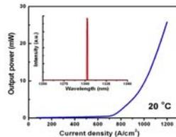
InAs/GaAs QD laser on Si substrate
